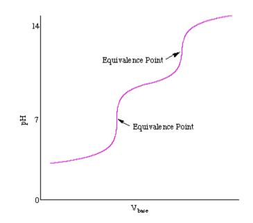
The titration bend appeared above is for a diprotic corrosive, for example, H2SO4and is similar to two stacked . For a diprotic corrosive, there are two buffering areas and two comparability focuses. This demonstrates the prior declaration that polyprotic acids lose their protons in a stepwise way.
