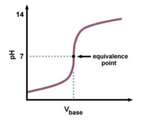
The titration of a solid corrosive with a solid base delivers the accompanying titration bend:
