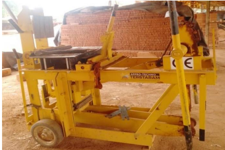
Figure 2: Picture of the manual press used for manufacturing the bricks
