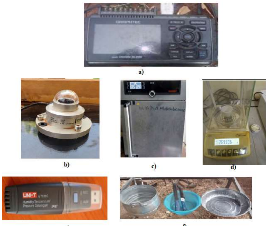
Figure 2: Images of measuring instruments (a: data logger, b: pyranometer, c: oven, d: balance, e: hygrometer, f: utensils)
