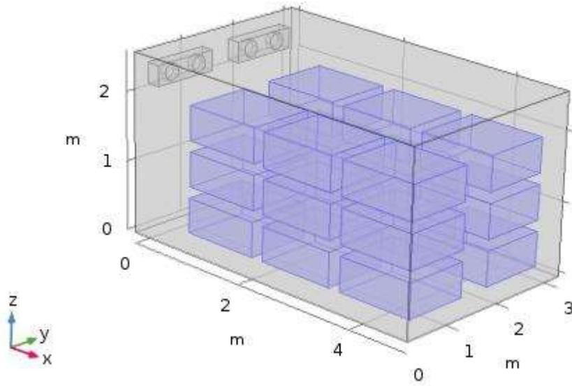
Figure 1: Model of the cold device containing the loaded products
