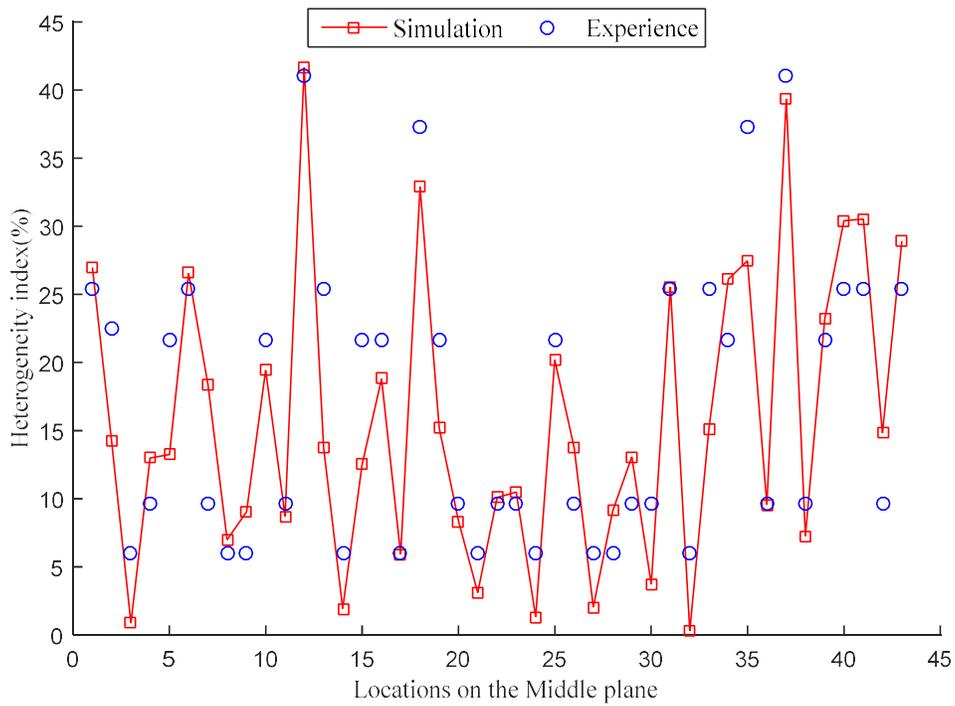
Figure 6: Comparison of simulated and experimental airflow profiles in the middle planes
