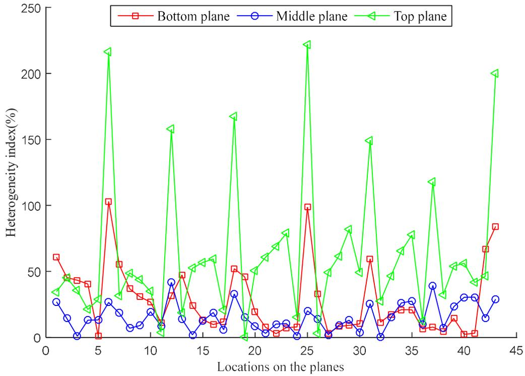
Figure 5: Air velocity heterogeneity index at 43 points on the different planes
