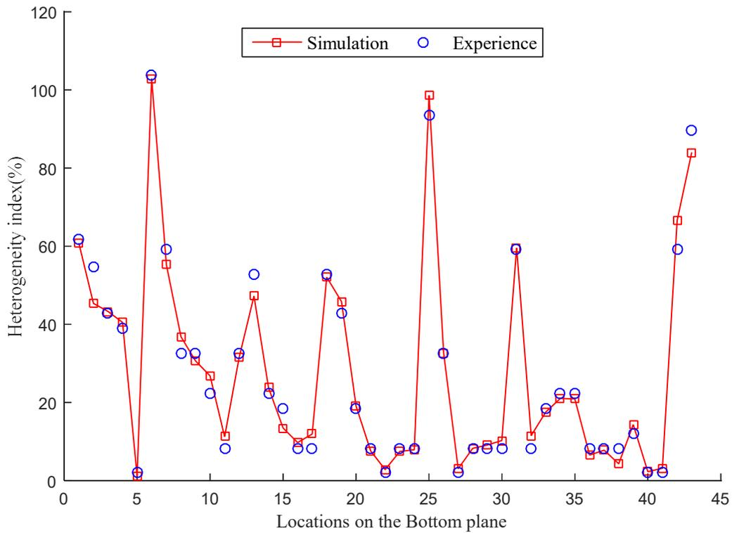
Figure 7: Comparison of simulated and experimental airflow profiles in the lower planes
